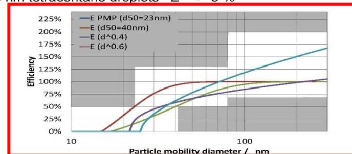
Figure 2: Schema of the limits for the number concentration efficiency curve (white area) and examples of efficiency curves conform to the requirements (curves)
