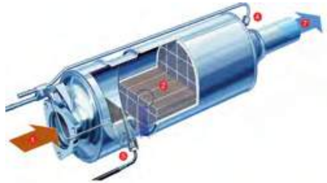
Diesel Particle filter DPF insulated in a steel case, with upstream DOC and control sensors; PEUGEOT 2000
