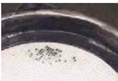
Small internal cracks are clearly visible by single black cells on the filter exit side
