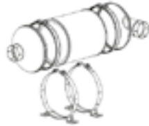
Fixation to the vehicle frame must respect the very high vibrations
