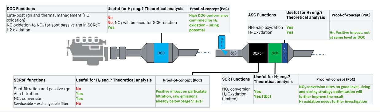
Achievement of the Stage V emission targets is feasible with the existing system layout. Impact on durability is under evaluation. To meet more stringent limits, further improvements are required.
