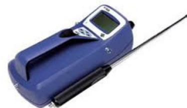
P-Track 8525: Condensation Particle Counter (CPC)
