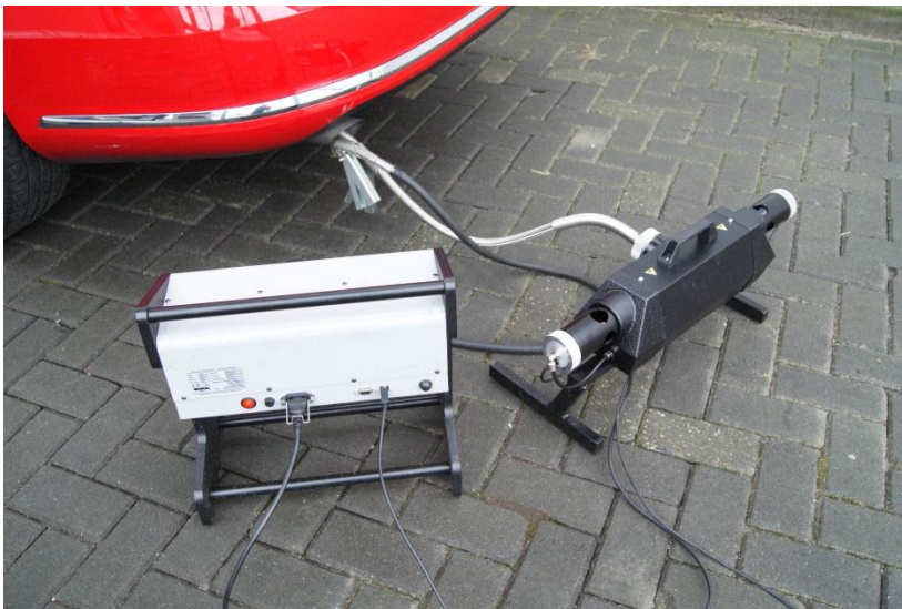
Research of a new PTI DPF PN emission test procedure
