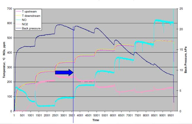
BPT of X25 NT1 after cleaning with Tunap cleaning fluid
