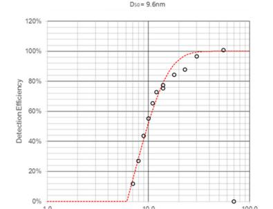
CPC-UT Standalone Detection Efficiency for Ts=36°C and Tc=20°C. classified miniCAST soot
