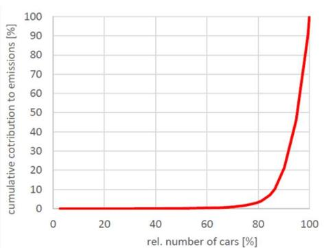
PN emission at low idle of 1000 diesel vehicles at Zürich 2018 with DPF [2]; 5% emit 80% of total PN
