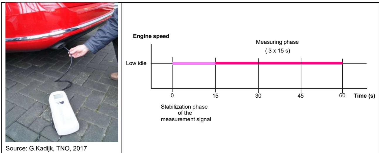
The particulate measurement can be performed regardless of the operating state (cold/warm, EGR valve open/closed) of the engine since a diesel engine with a faultless filter usually emits significantly less than 3'000 1/cm<sup>3</sup> at low idle, i.e. much less than what is set as the limit for passing the test (see section 5). There is therefore no need to condition the engine before the test procedure.
